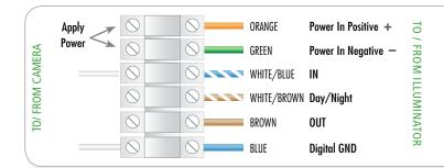
To switch illuminator ON, your camera output port(s) have to be ACTIVE and set to LOW (GND-ground).
