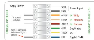
To activate desired angle the corresponding output on the external controller must be set to active low.
