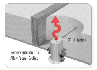
3. Remove at least 3" of insulation around the light to allow proper cooling. If necessary use a recessed light draft stop cover.
