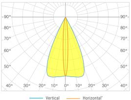
Note: \*The above color key is for a Linear light mounted vertically. For a horizontally mounted light, the colored lines would represent the reversed.
