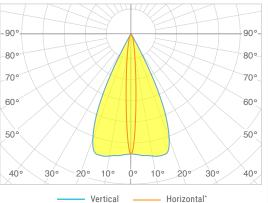
Note: "The above color key is for a Linear light mounted vertically. For a horizontally mounted light, the colored lines would represent the reversed.
