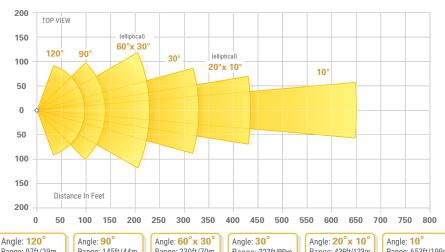
Range: 97ft/29m HFOV: 168ft/51m Range: 145ft/44m HF0V: 184ft/56m Range: 230ft/70m HFOV: 230ft/70m
