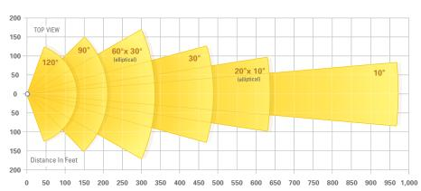
Angle: **120°** Range: 145ft/44m HF0V: 251ft/76m Angle: 90° Range: 211ft/64m HFOV: 272ft/83m Angle: **60°x 30°** Range: 344ft/105m HF0V: 344ft/105m
