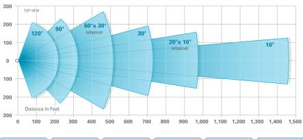
Angle: **120°** Range: 223ft/68m HFOV: 387ft/118m Angle: **90°** Range: 327ft/99m HFOV: 420ft/128m Angle: 60°x 30° Range: 508ft/156m HFOV: 508ft/156m
