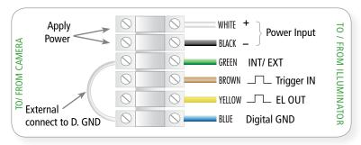
You will need to log into the appropriate software interface and program the I/O ports to trigger when flash is desired.
