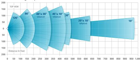
Angle: 120° Range: 145ft HF0V: 251ft Angle: 90° Range: 211ft HFOV: 272ft Angle: 60°x 30° Range: 344ft HFOV: 344ft Angle: 45°x 10° Range: 450ft HFOV: 346ft Angle: 30° Range: 484ft HFOV: 250ft Angle: 20°x 10° Range: 641ft HFOV: 200ft Angle: 10° Range: 968ft HFOV: 169ft
