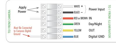
To switch illuminator ON, your camera output port(s) have to be ACTIVE and set to LOW (GND-ground).
